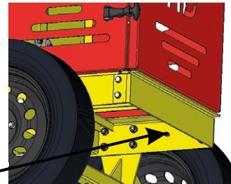
Grounding point in the machine.
