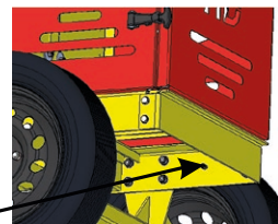
Grounding point in the machine.
