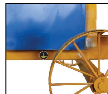
Concrete mixer grounding point.
